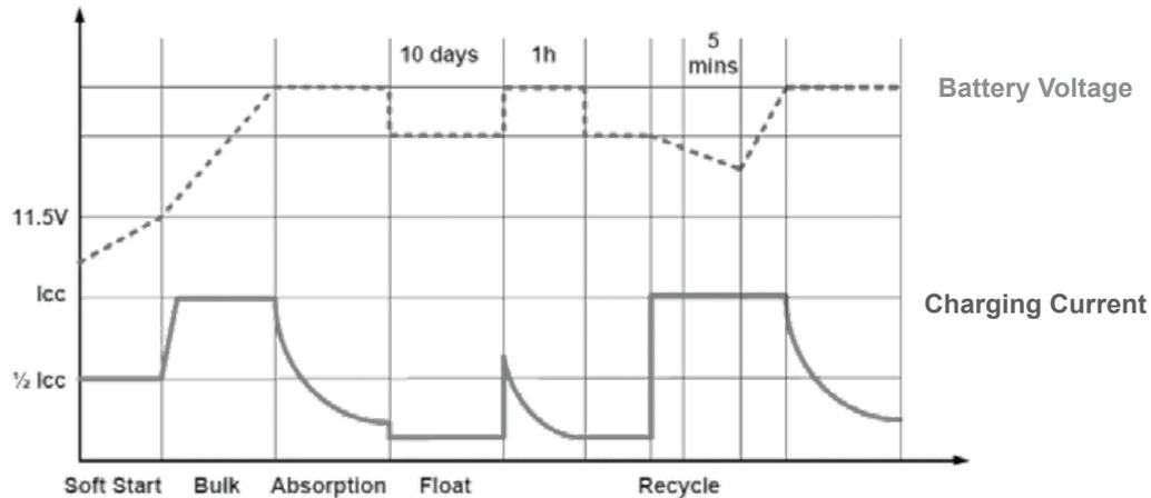
**Soft Start(Stage 1)** – The controller will deliver  $\frac{1}{2}$  rated current until the battery voltage is over 11.5VDC or 10-minute time-out, then turn to the Bulk(Boost) Stage.
