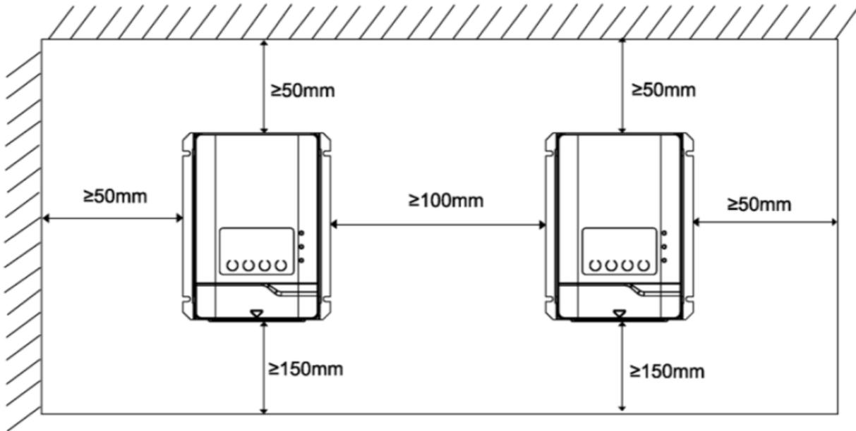
Please choose a flat and clean surface for installation, mark the position for the 4 mounting point and use the 4 x M5 mounting screw sets supplied. Please tighten the screws properly and make sure all 4 screws are installed to avoid falling. Install the SC520/SC540 as close to the batteries as possible. This will reduce the potential for voltage drop and ensure maximum performance of the equipment.
