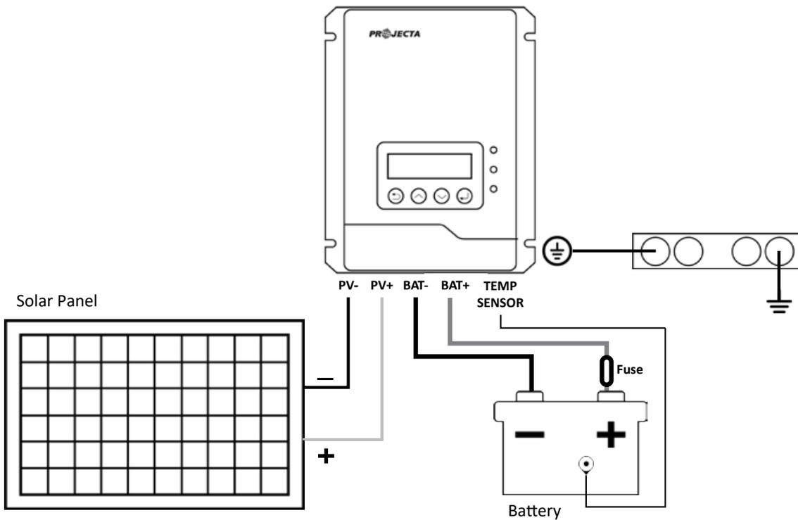
1. Connect the positive battery wire followed by the negative battery wire.
